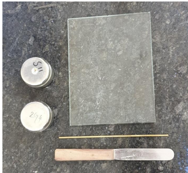
Figure 1: Equipment for Plastic Limit
