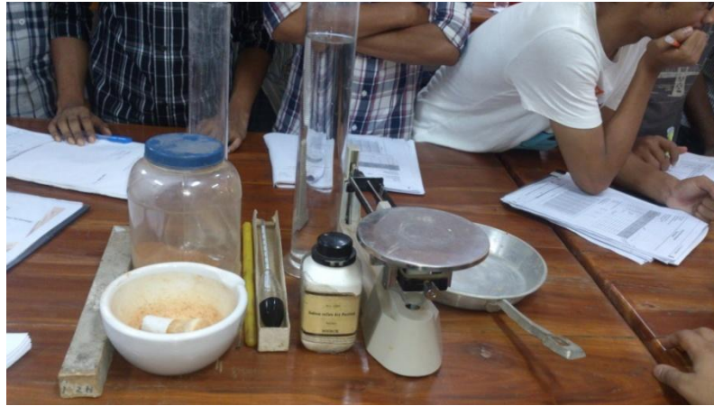
Figure 4.2 Hydrometer Test Apparatus
